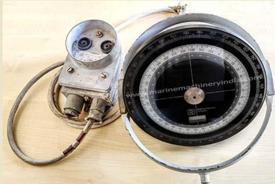
Figure 1 Raytheon Anschutz 133-407.NG001 bearing repeater compass with dimmer and setting switch
