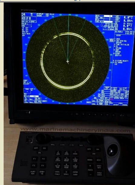
Figure 24 Test result for Performance Monitor function
