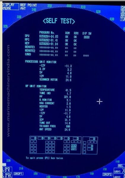
Figure 25 Furuno FAR-2117 radar Self Test result - 1
