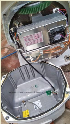
Figure 111 Furuno RSB-096 with performance monitor - inside mechanism 3
